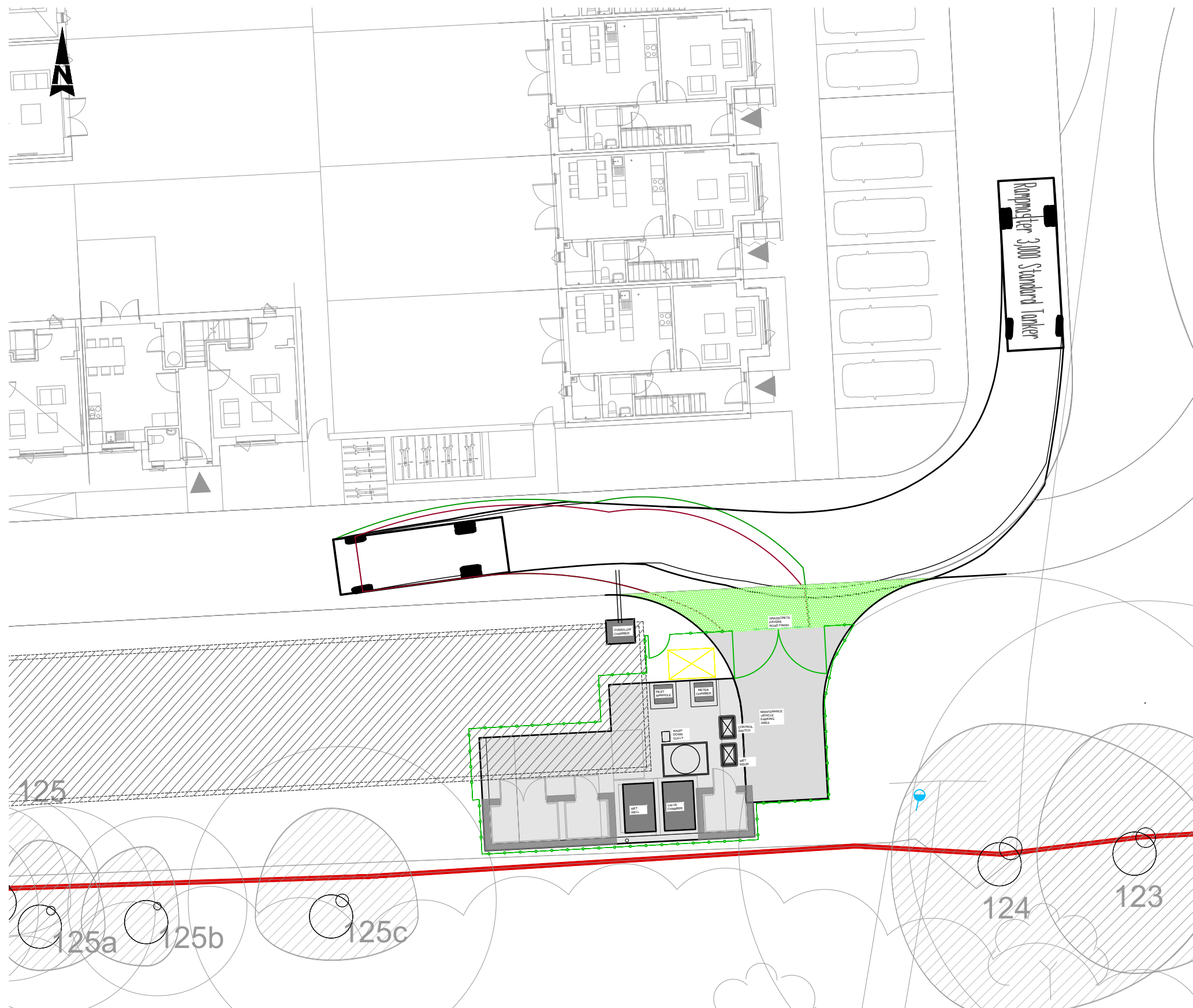
FOUL PUMPING STATION AND 24 HOUR EMERGENCY STORAGE TANK (732m³)
